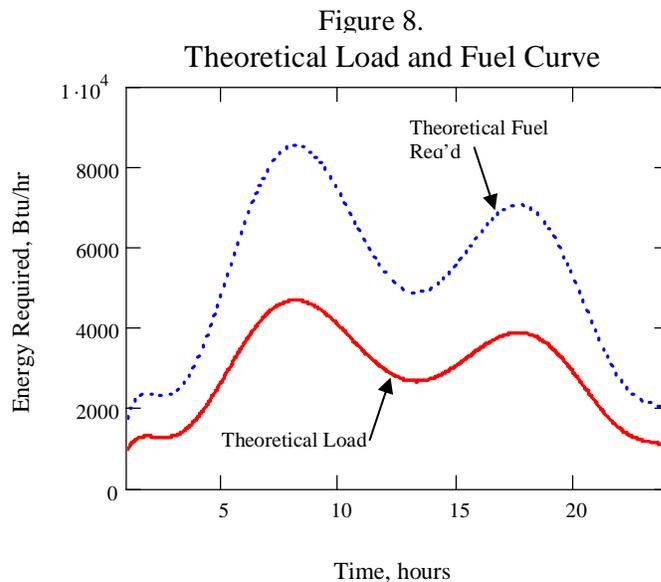
The theoretical fuel required at anytime during this 24-hour cycle is much greater than the actual load requirement. In this case, system efficiency is approximately 55%. The challenge to the facilities manager is to bring the *Fuel Required* curve closer to the *Theoretical Load* curve.
